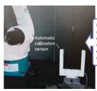
Preventive maintenance against torch displacemen can be performed by running the displacement detection program at regular intervals.
