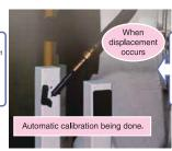
If displacement is detected the calibration program is automatically run for correction. The task program is automatically modified. Hardware
